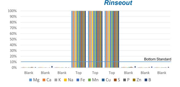
The SampleSense Soil rinseout immediately reduces all elements to concentrations well below the bottom standard when using the six second Mehlich-3procedure. Additional seconds can be added to the rinse-out to meet lab requirements. The system can deliver rinse-out factors of 1,000x, 10,000x or more depending on how clear the spray chamber needs to be before the next sample is introduced.
