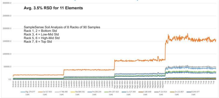
Analysis of 720 samples in 70 minutes. The four levels represent two racks of 90 samples, with each of the four calibration standards levels individually loaded with 5 mL of liquid into each of the 90 positions contained in each set of racks. Excellent stability observed from within each of the four concentration levels.
