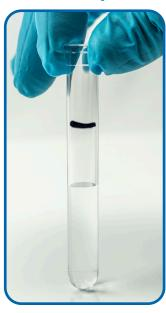
SampleSense Soil consumes < 2 mL of sample. The black line shows the original level of 5 mL extract. Post analysis 3.5 mL remains. Samples can be reanalyzed without re-extraction
