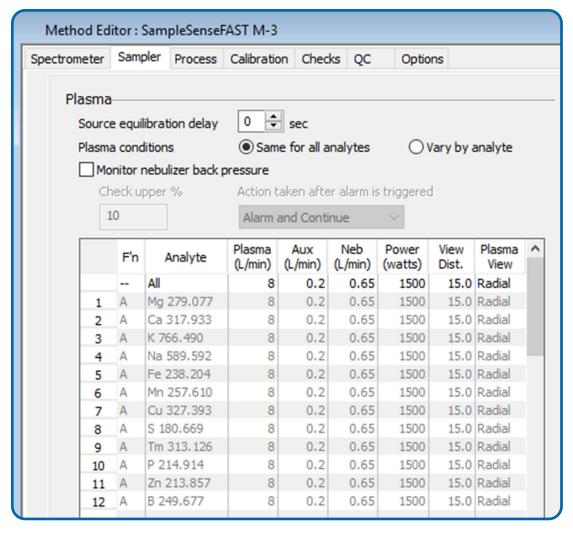
PerkinElmer Optima 8300 ICP method conditions
